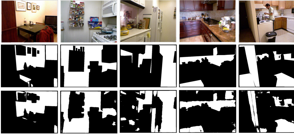
Figure 4.5: Visualization of segmentation results of "kitchen" (scene 1 in experiment 1), top row: real image, middle row: ground truth segmentation, bottom row: segmentation generated by EWC. White: background, Black: foreground.
